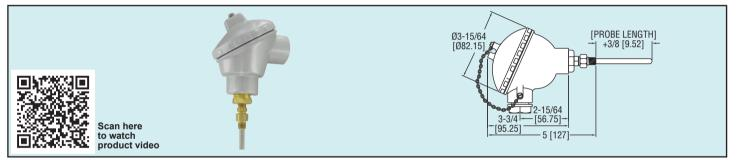
**The Series TTW Immersion Temperature Transmitter** combines three popular products into a single package. Our TBU series head mounted temperature transmitter is factory mounted into our A-709 enclosure. A Pt100 RTD version of our TE series is wired to the transmitter, giving insertion lengths up to 18<sup>°</sup>. Each transmitter is factory programmed and calibrated to output a 4 to 20 mA signal proportional to the 32 to 212°F (0 to 100°C) temperature range.
